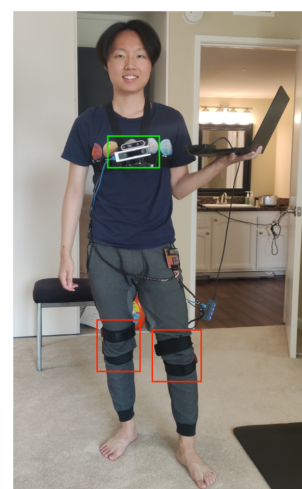
Figure 3: Original setup with two Realsense cameras (green) and four IMUs (red)
