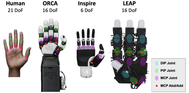
Fig. 1. Comparison of joints in the human hand to the ORCA, Inspire, and LEAP hands. The MCP Abd/Add for the thumb is also the CMC joint.
